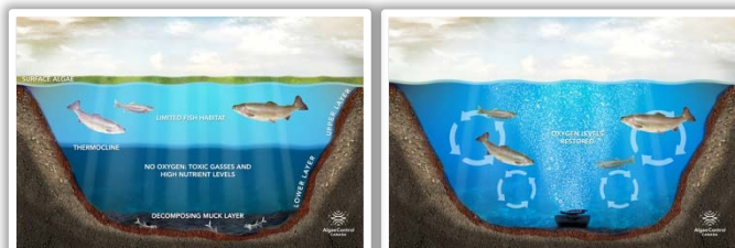
The aerated pond on the right has oxygen throughout the water column (images courtesy of Algae Control Canada).
