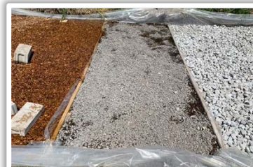
Three 'cells': woodchips, slag, and gravel.
