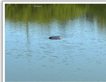
A sonication unit in a treatment pond.
